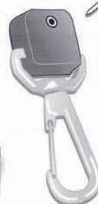
■ Add-A-Clip® Stainless Steel Threaded Stud penetrates webbing or material (tabs, flaps, pockets), screws into Add-A-Clip housing for a secure mount. Available in multiple configurations
